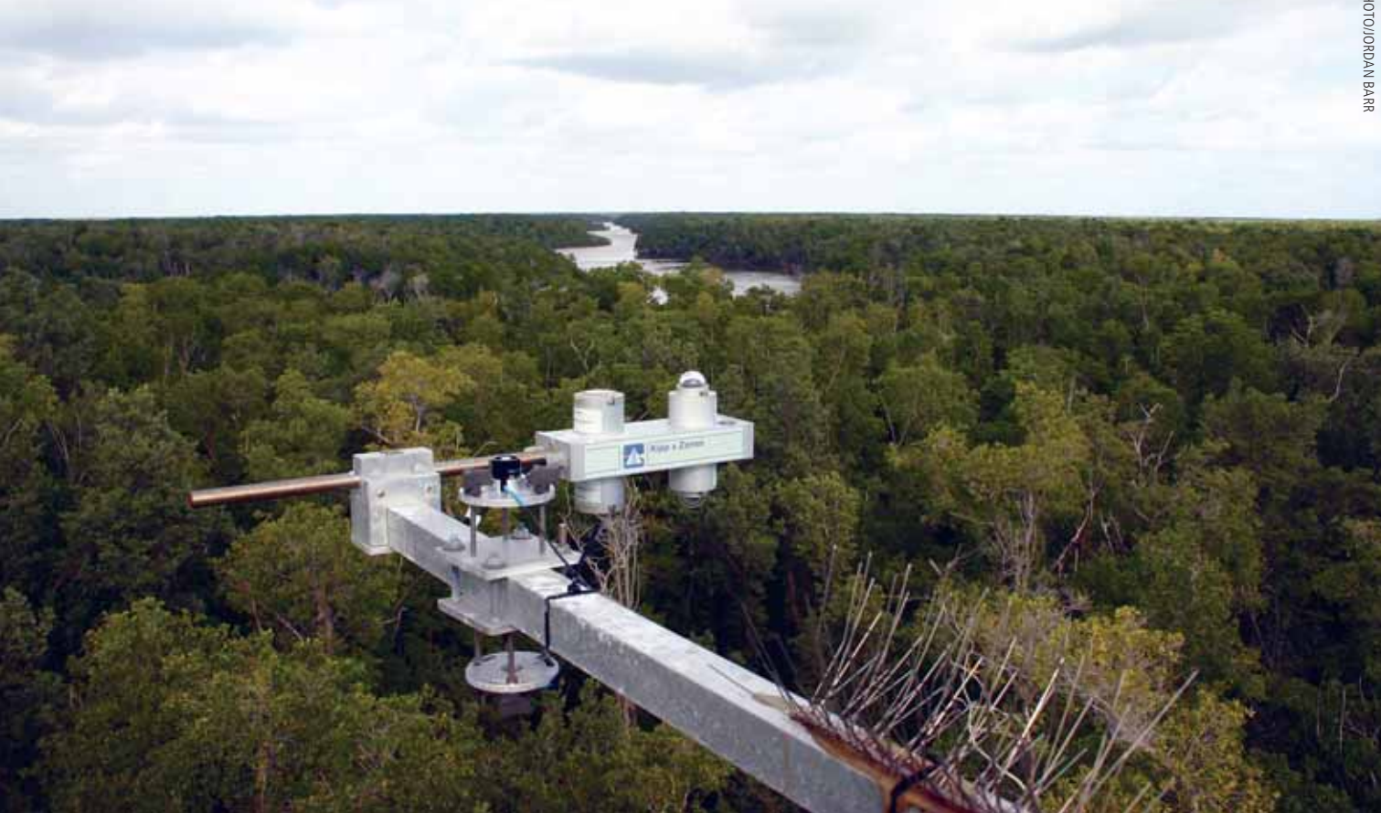
Figure 6. Resource managers measure irradiance above a mangrove forest through the use of net radiometer and up- and down-facing quantum sensors mounted on a tower at 90 feet (27 m). Irradiance is one factor, along with atmospheric carbon and other physical factors, that influences the cycling of carbon through the mangrove ecosystem. Shark River is visible in the distance. This tower is associated with the project to measure carbon dynamics in mangrove forest.
